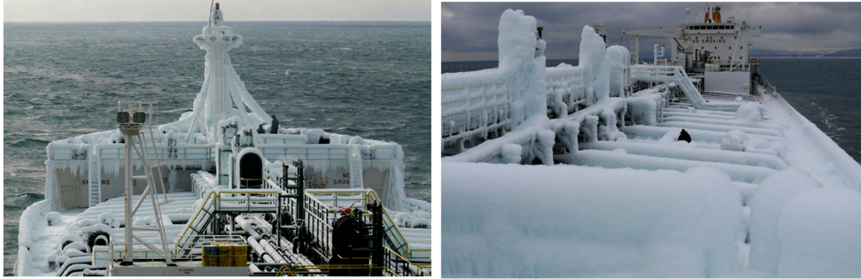
Figure 1.5: Severe icing of cargo vessel superstructure from sea spray in the port of Quebec. Reprinted from Dehghani-Sanij et al. (2017), with permission from Elsevier.
