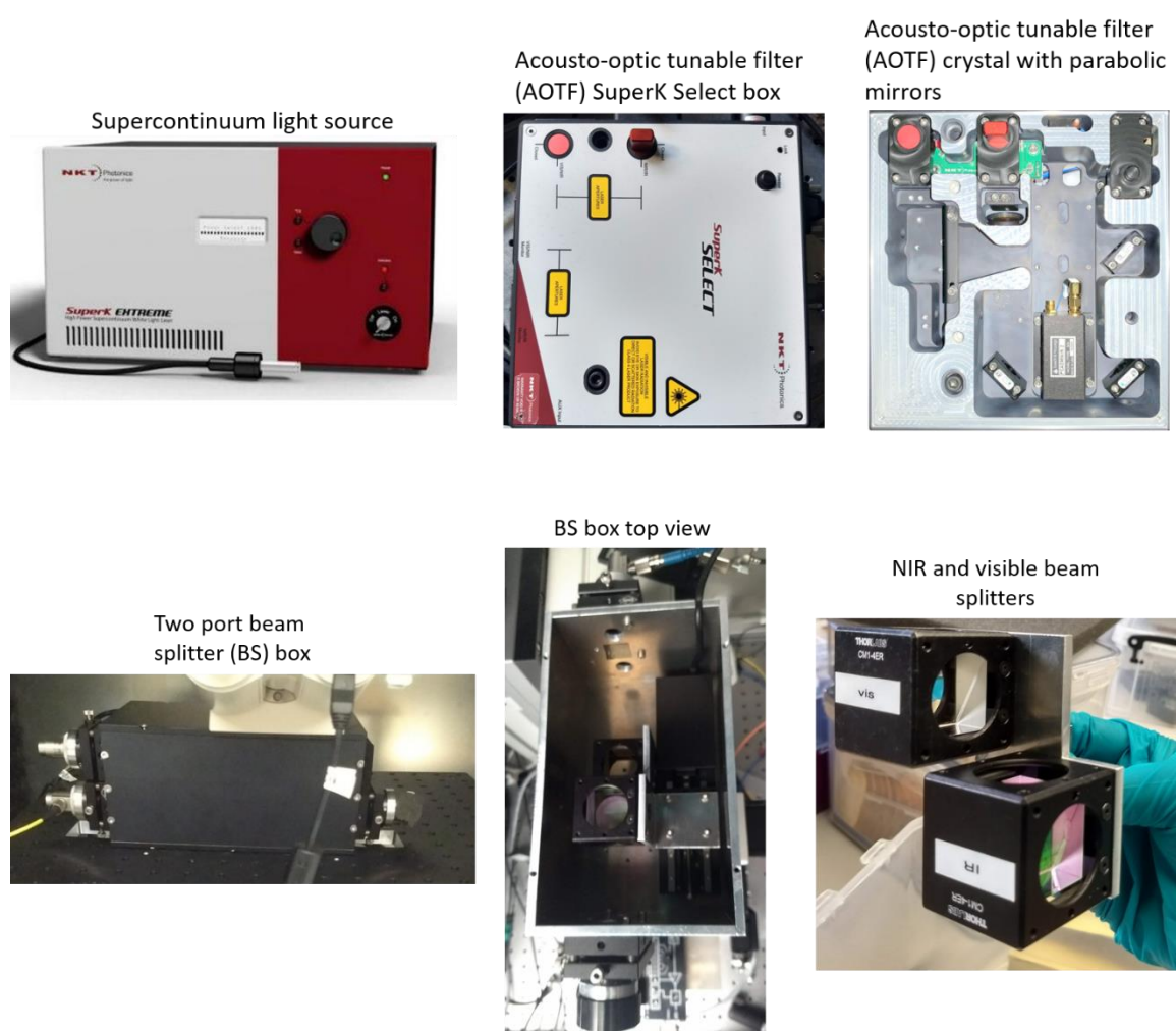
Figure 3.3: Photocurrent setup components that include supercontinuum light source, acousto-optic tunable filter, beamsplitters. AOTF photograph by P. B. Selvasundaram.
