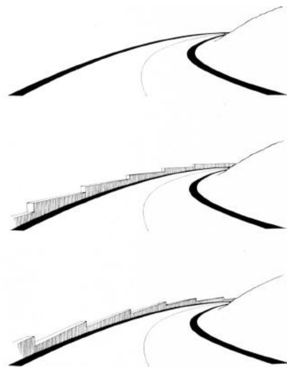
Figure 3.52 - Influence on marginal elements on road perception, misunderstanding of the slope. From Lorenz (Lorenz, 1971)
