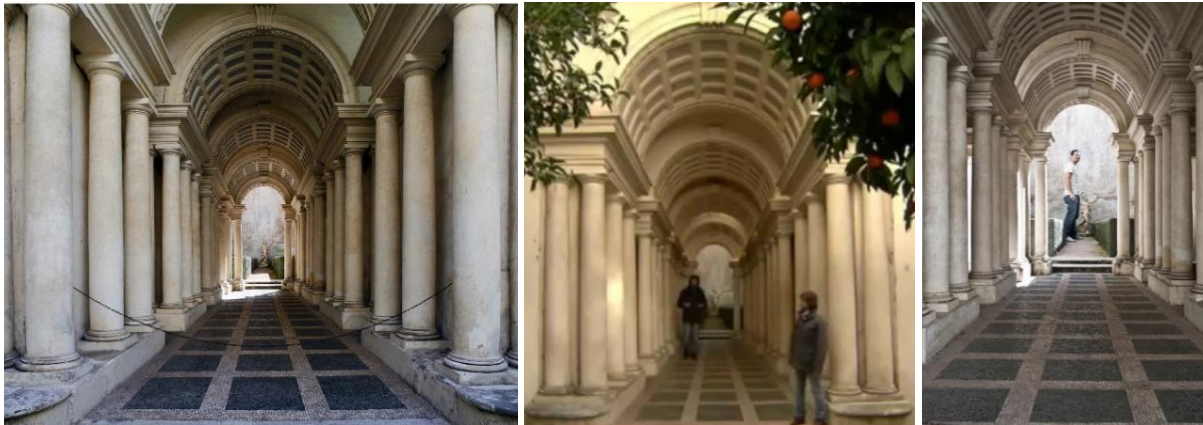
Figure 3.46 – Example of distance and dimensions optical illusion from the Borromini Gallery in Rome. The columns and the geometrical reference of the pavement seem to be of the same dimension, but they are not. This creates the perception of a long tunnel and a big sculpture in the end 9
