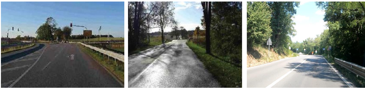
Figure 3.54 – Examples of invisible or not clear PCLs: left - intersection where the main road goes straight (Birth, 2004), center – intersection not visible 125 m ahead (Birth, 2004), right – pedestrian crossing not visible 50 m ahead (photo by Andrea Paliotto)
