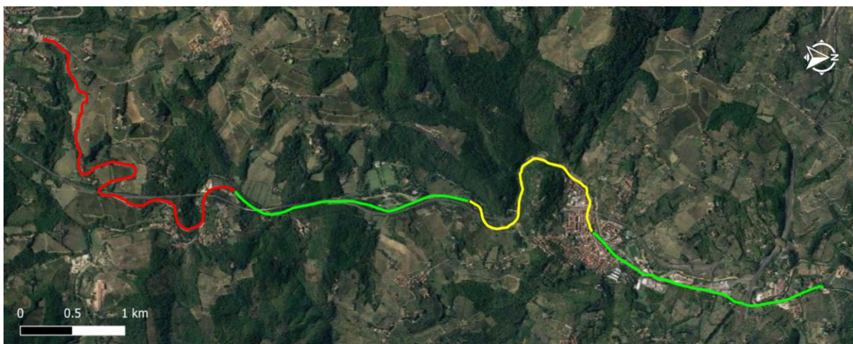
Appendix Figure 12 – SR2, stretches with the same CCR on satellite image (red= high CCR, yellow = medium CCR, green = low CCR)
