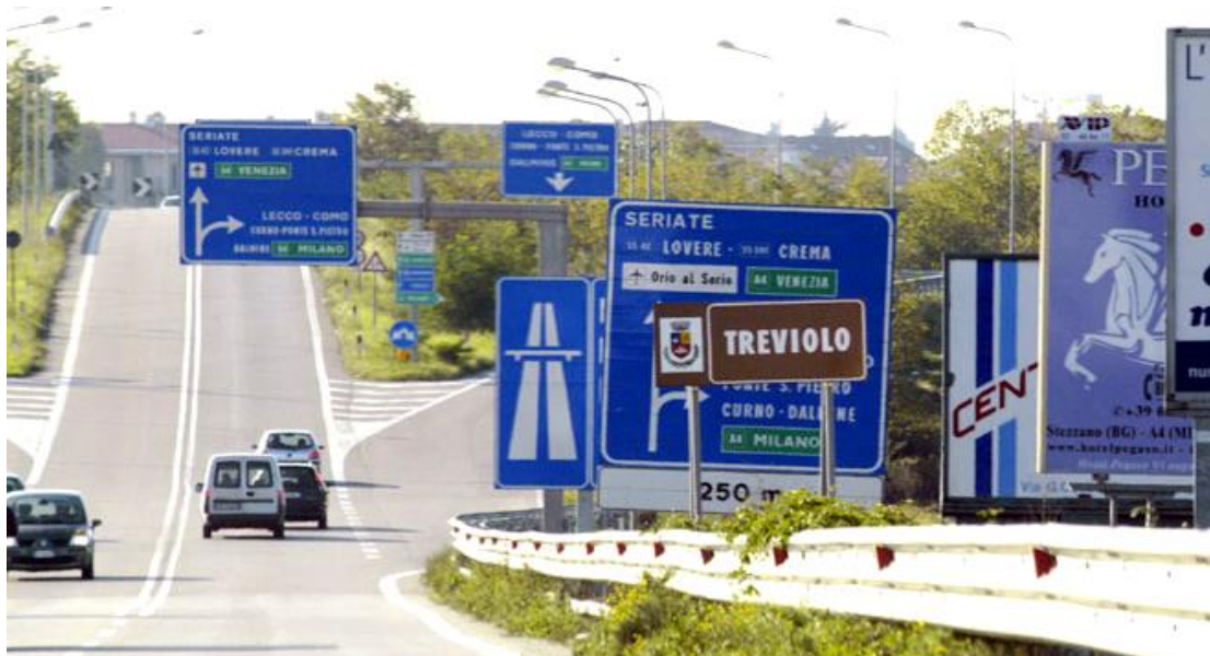
Figure 3.59 – Bad positioning and overload of information provided by vertical signs
