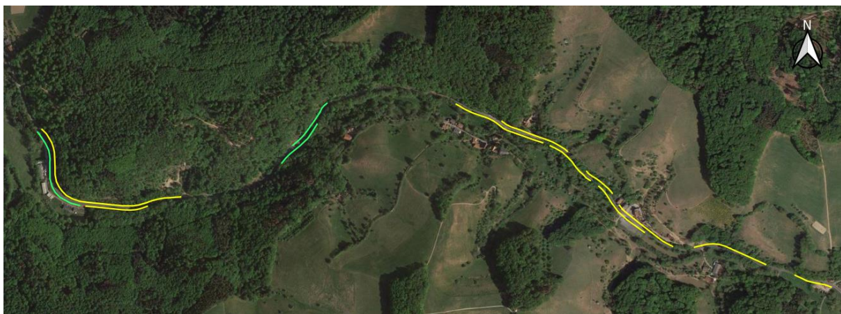
Figure 6.45 – Total HFS results, L3408 (yellow = medium risk HFES, green = low risk HFES)
