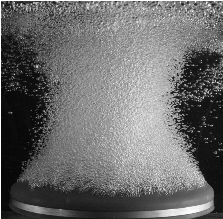
Figure 6: Hourglass shape of a bubble swarm
