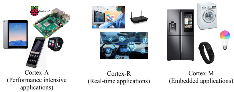
Figure 14: IoT device classes from ARM Cortex family in decreasing order (left to right) of their sizes and processing capabilities, and respective application examples.
