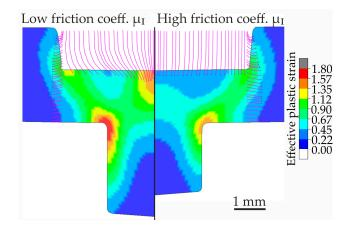
**Figure 11.** The comparison of a low and high friction coefficient  $\mu_I$  (c.f. Table 1) between the punch and steel blank during pin extrusion.
