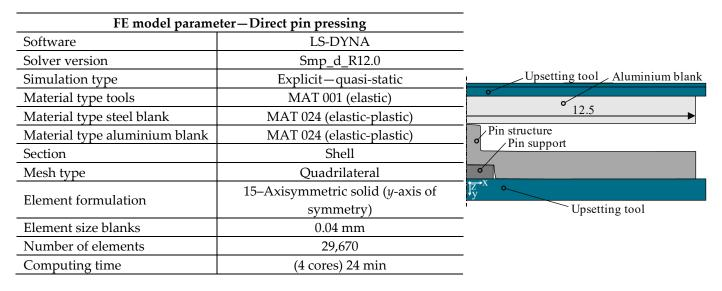
**Figure 7.** The relevant parameters of the FE-simulation of the direct pin pressing process as well as the FE-model design with the initial dimensions.
