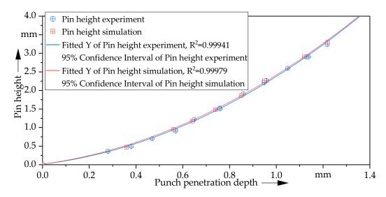
**Figure 5.** The comparison of the experimentally measured pin heights and punch penetration depths with the pin heights and punch penetration depths determined with the described numerical simulation. Both data sets were fitted with a 2nd grade polynomial to ensure better comparability.
