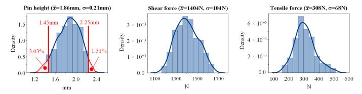
Figure 13. Property distribution of pin joint characteristics based on the second robustness analysis.
