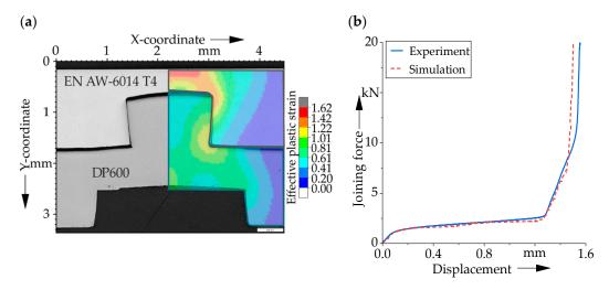
**Figure 8.** (a) The comparison of the geometric properties of a direct pin pressing joint using a micrograph of a pin with a height, *h*, of 1.38 mm from a sheet of DP600 with a thickness of  $t_0 = 1.5$  mm and an aluminium joining partner of EN AW-6014-T4 with a thickness of  $t_0 = 1.5$  mm, and the results of the numerical simulation with corresponding parameters. (b) Numerically determined and experimentally measured force-displacement curves for direct pin pressing.
