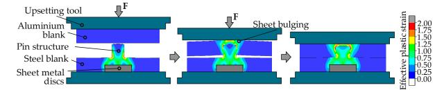
Figure 3. Illustration of the direct pin pressing joining strategy.
