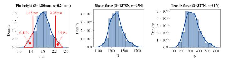
Figure 12. Property distributions and failure probability of pin joint characteristics.
