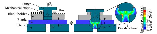
Figure 2. Illustration of the pin extrusion process and relevant process parameters.
