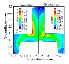
**Figure 6.** Comparison of the effective plastic strain with the microhardness measurement of a pin with a height of 2 mm and a diameter of 1.0 mm.
