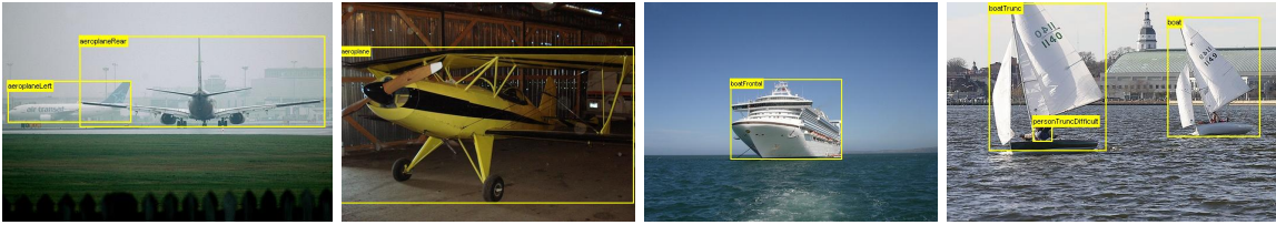
Figure 1.2: Examples of high intra-class variation. The aeroplane class shows instances of passenger plane and propeller-driven aircraft, while the boat class includes cruise ships and sail boats. This intra-class variation causes a high variation of the appearance of different object instances. The yellow boxes show the original annotations.
