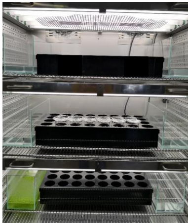
Figure 10: Schematic of the plant growth cabinet incl. the black storage boxes.
