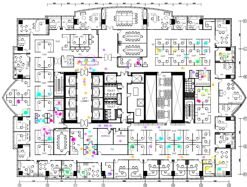
Figure 6.46: Activity Sampling during office-hour of Planning Department in Organisation A (22 nd Floor)
