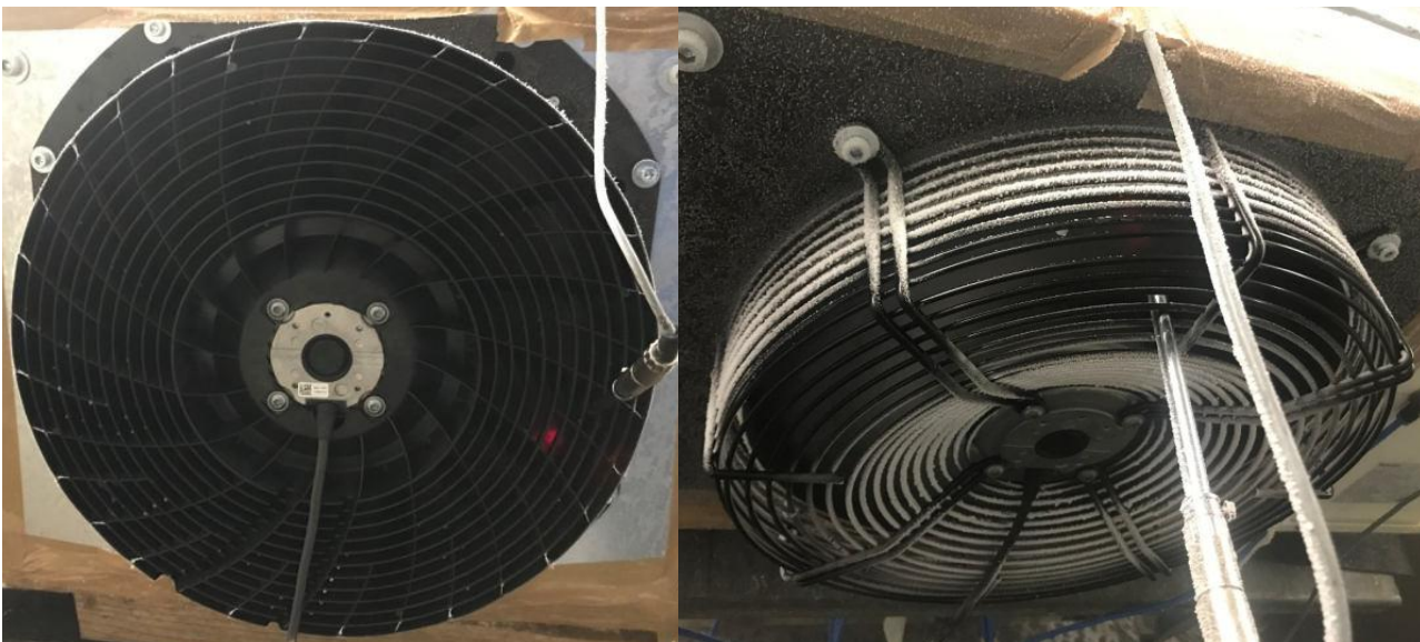
Figure 8: icing test result of the new fan (left) vs. the baseline fan (right) [2]
