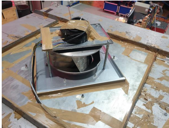
Figure 7: Experimental test setup using plenum chamber
