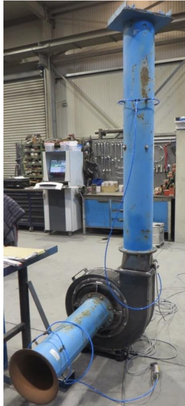
Figure 4: test stand for fan TES14-200
