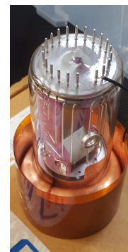
Figure 7. Electrostatic shielding wrapped around the PMT.
