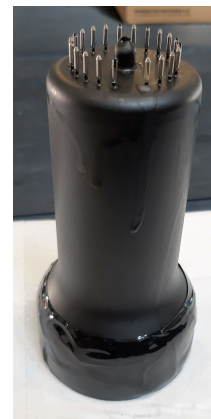
Figure 9. Fully treated PMT with protective foil.
