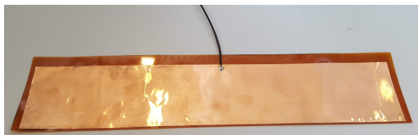
Figure 6. Electrostatic shielding in the expanded form.
