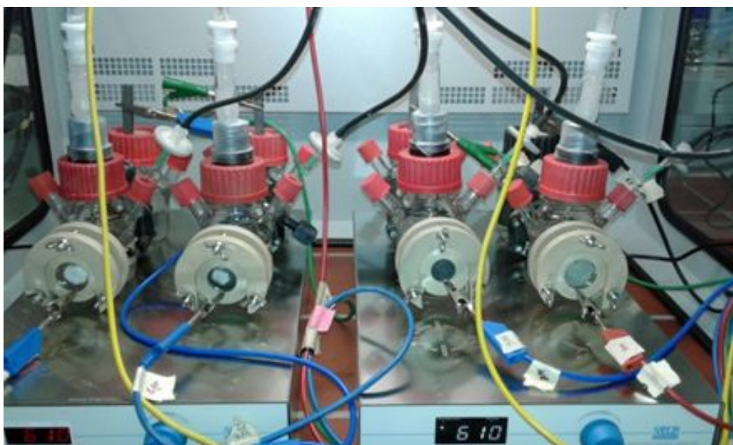
Figure S6: MFCs connected to a multipotentiostat placed on multi-position magnetic stirrer inside an incubator.
