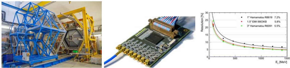
Figure 5. ECAL frame (left), the PaDiWa-AMPs read-out board (middle) and lead glass module resolution as a function of the incident photon energy (right).
