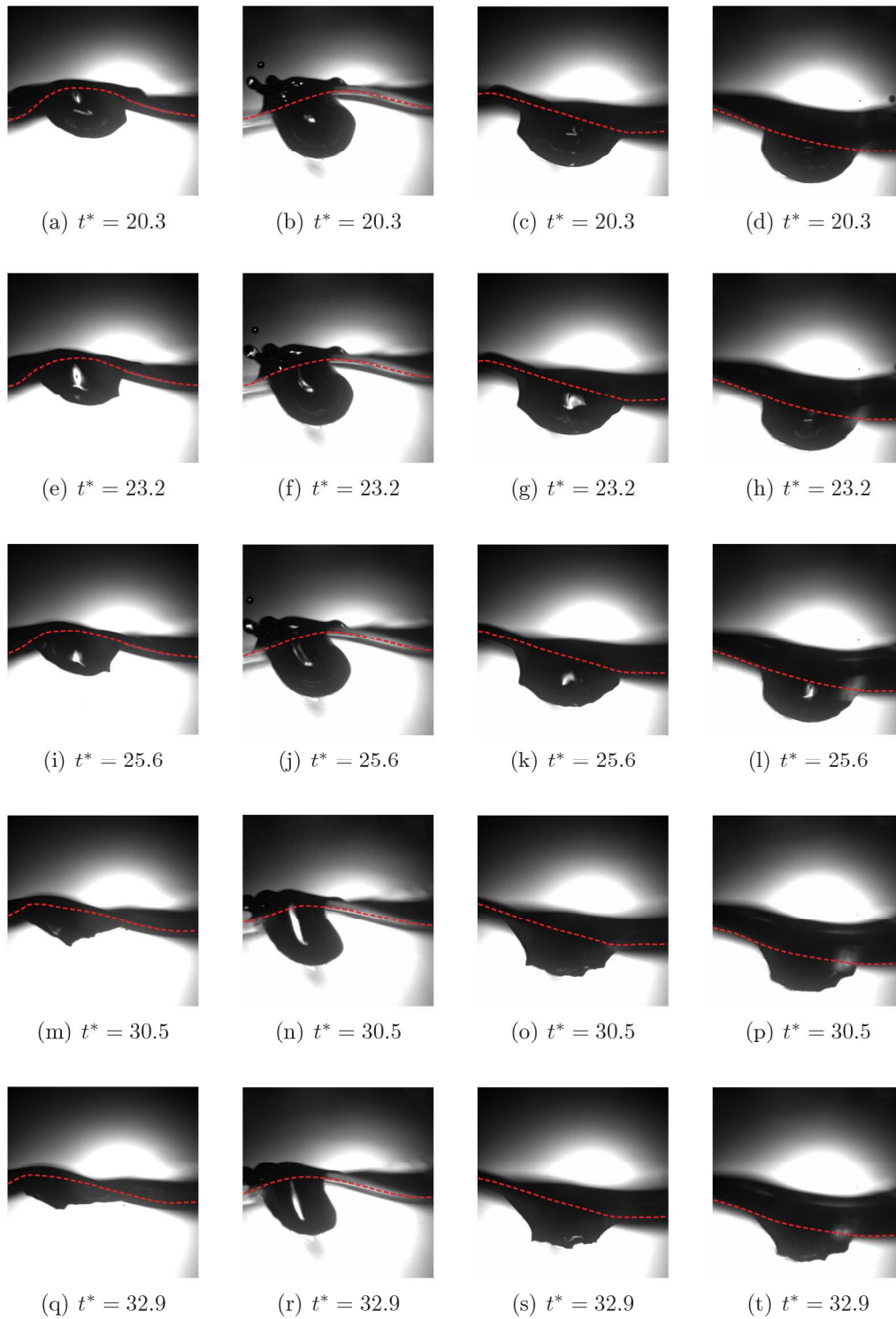
Figure 5.13: The evolution of the cavity formed by single drop impingement onto a solitary wave at \varphi = 60^\circ and \varphi = 147^\circ for distilled water and a glycerine/water mixture at non-dimensional time instants between t^* = 20.3 and t^* = 32.9 . The impingement parameters are: U_d = 3.0 m/s, D_d = 2.9 mm and U_w = 0.4 m/s (distilled water) and U_d = 3.0 m/s, D_d = 2.6 mm and U_w = 0.3 m/s (glycerine/water). Outer left: \varphi = 60^\circ ( We = 354 , Fr = 339 , Re = 10,421 ); Middle left: \varphi = 58^\circ ( We = 413 , Fr = 443 , Re = 10,944 ); Middle right: \varphi = 147^\circ ( We = 342 , Fr = 348 , Re = 10,093 ); Outer right: \varphi = 144^\circ ( We = 333 , Fr = 361 , Re = 9,813 )
