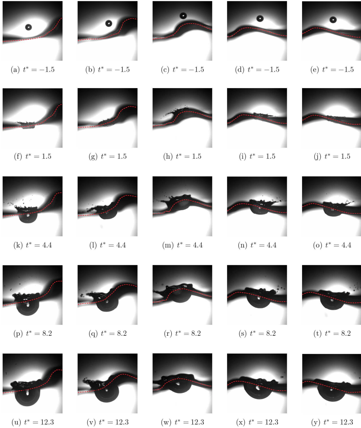
Figure 5.3: Single drop impingement onto different phases of the solitary wave between \varphi = 1^\circ and \varphi = 147^\circ . The evolution of the cavity formed by a distilled water drop impingement at non-dimensional time instants between t^* = -1.5 and t^* = 12.3 . The impingement parameters are for all shown phases: D_d = 2.9 mm, U_d = 3.0 m/s and U_w = 0.4 m/s. Outer left: \varphi = 1^\circ , We = 335 , Fr = 346 , Re = 9,947 ; middle left: \varphi = 21^\circ , We = 331 , Fr = 349 , Re = 9,845 ; middle: \varphi = 60^\circ , We = 354 , Fr = 339 , Re = 10,421 ; middle right: \varphi = 125^\circ , We = 352 , Fr = 351 , Re = 10,299 ; outer right: \varphi = 147^\circ , We = 342 , Fr = 348 , Re = 10,093
