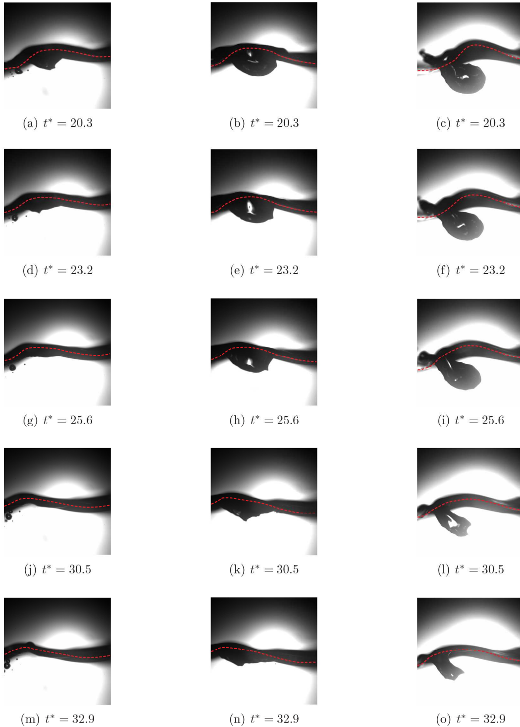
Figure 5.7: Single drop impingement onto a solitary surface wave for different drop impingement Weber numbers. The evolution of the cavity formed by a distilled water drop impingement at non-dimensional time instants between t^* = 20.3 and t^* = 32.9 . The impingement parameters are (left) D_d = 2.9 mm, U_d = 2.7 m/s, U_w = 0.4 m/s and \varphi = 60^\circ ( We = 256 , Fr = 282 , Re = 8,552 ); (middle) D_d = 2.9 mm, U_d = 3.0 m/s, U_w = 0.4 m/s and \varphi = 60^\circ ( We = 354 , Fr = 339 , Re = 10,421 ) and (right) D_d = 2.9 mm, U_d = 3.2 m/s, U_w = 0.4 m/s and \varphi = 56^\circ ( We = 400 , Fr = 391 , Re = 11,024 )
