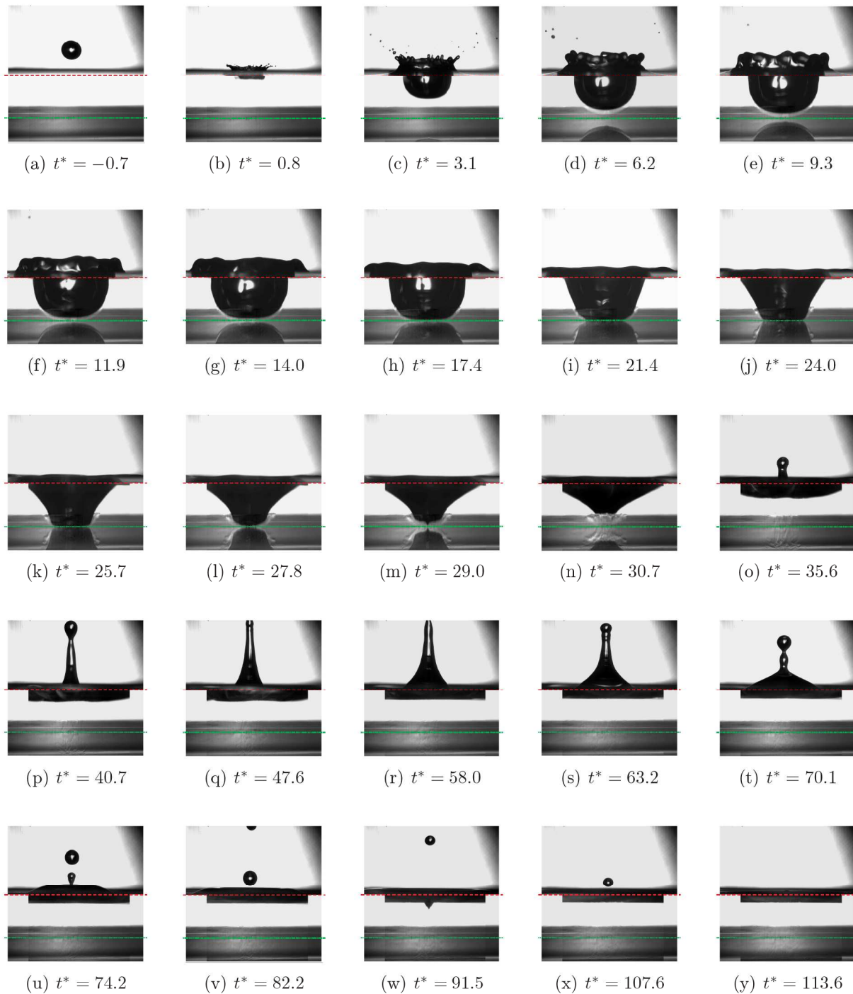
Figure 4.1: Single drop impingement onto a liquid layer of non-dimensional thickness h^* = 2 . The evolution of the cavity formed by a distilled water drop ( We = 350 , Fr = 273 , Re = 8,931 ) impingement at various non-dimensional time instants. The impingement parameters are D_d = 3.1 mm and U_d = 2.9 m/s
