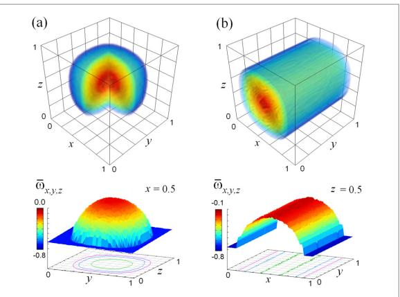
**Figure 3.** Spatial profiles of average frequencies for an incoherent ball (left panel) and an incoherent tube (right panel). Equation (2) was integrated up to  $T = 10\ 000$ , then averaging was calculated at the time interval  $\Delta T = 100$ . Parameters are the same as in figures 2(a) and (b), respectively.
