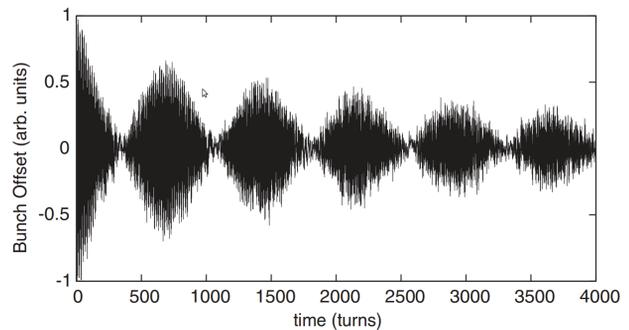
Figure 1: Recorded turn-by-turn beam oscillation in the vertical plane at SIS 18.
