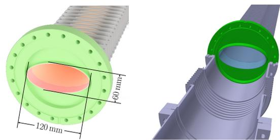
Figure 1: The dipole chamber on the left shows the smallest cross section of the beamline. The right image illustrates a typical step that occurs at the transition of two different pipe geometries.
