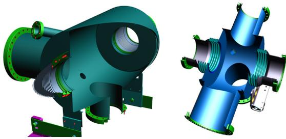
Figure 2: On the left a diagnostic chamber with a stair height of 90 mm at its entrance and its exit is displayed. The right image shows a pump chamber, which has one of the largest gaps in the SIS100 vacuum system that must be traversed by the inspection robot.
