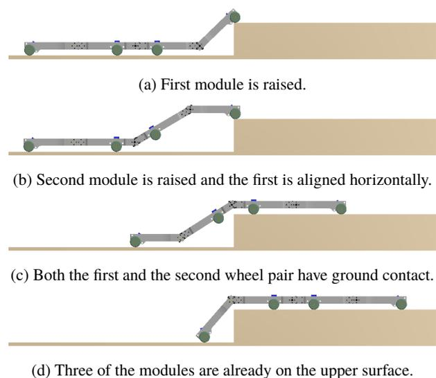
Figure 5: Movement sequence of climbing on a higher ground level for a robot with four modules.
