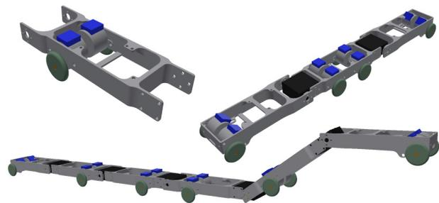
Figure 3: CAD model of the modular robot. On the top left, an example of a single module is displayed. The model on the top right shows the minimum robot configuration of three modules. The robot below consists of six modules.
