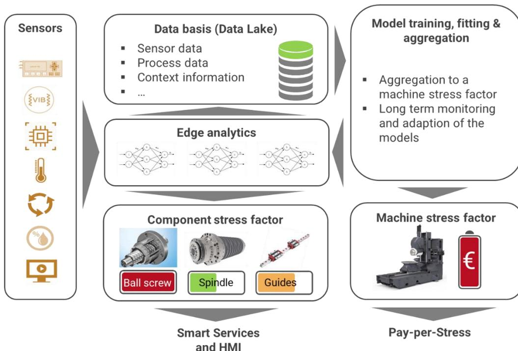
Figure 7: Concept for the development of a stress factor for stress-based payment models in machine tool industry
