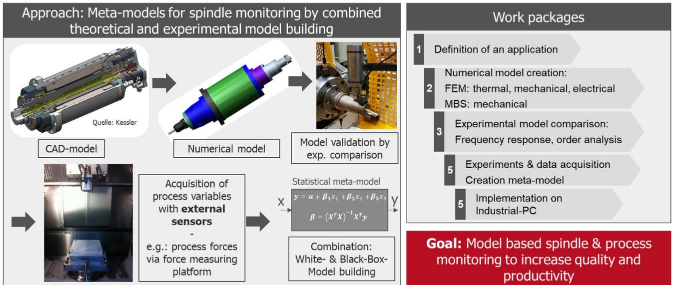
Figure 9: Procedure for model-based spindle monitoring
