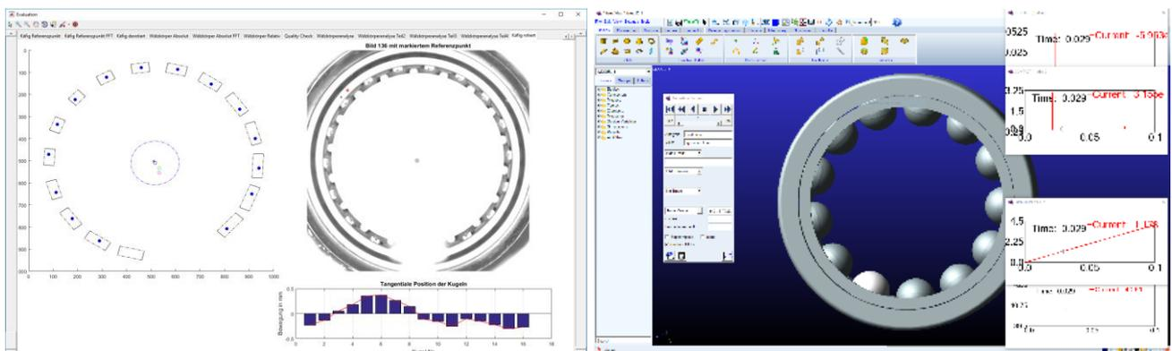
Figure 10: Optical measurement and modeling of unstable rolling bearing motion behaviour
