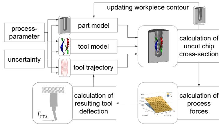
Figure 4: Framework of the mechanistic process model for tapping<sup>5</sup>
