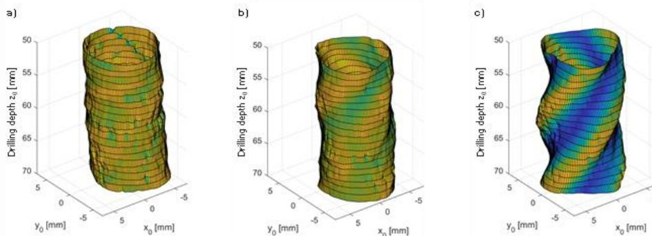
Figure 5: Representation of the experimentally determined bore wall for different guide chamfer widths (deviation from the ideal circular diameter enlarged by a factor of 50) a) 740 µm b) 500 µm c) 300 µm
