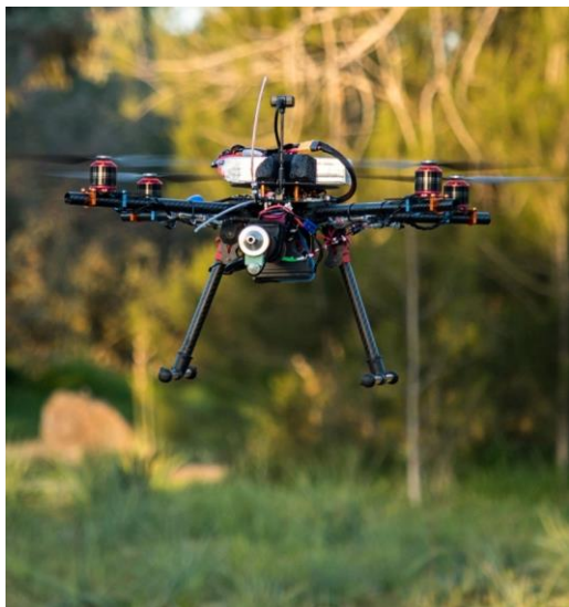
Figure S4. The tarot 650 quadcopter performing PM vertical profiles during an intensive campaign at CyI's premises in Nicosia on 28 February 2020.
