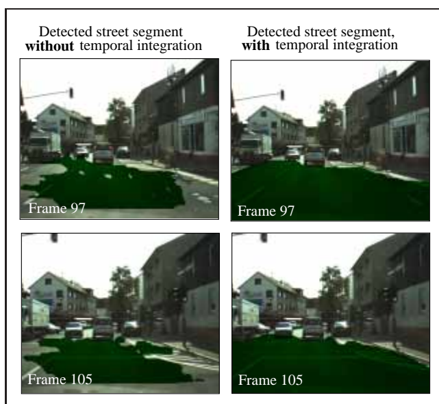
Figure 5: Road detection on example images of an inner city stream (left column: Without temporal integration, right column: With temporal integrated road segment).
