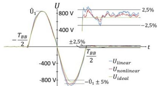
Figure 4: Linear and nonlinear predistortion for  $\hat{U} = 820$  V
