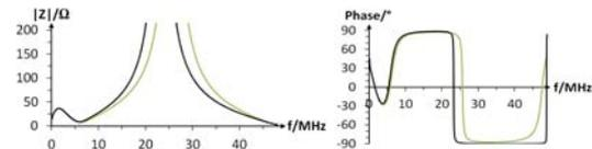
Figure 3: Impedance, comparison between measurement and simulation.
