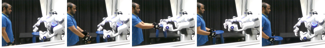
Figure 4.3.: Sample Human-Robot Interactions generated with the reactive motions generated by MoVEInt for a Bimanual Handover scenario.
