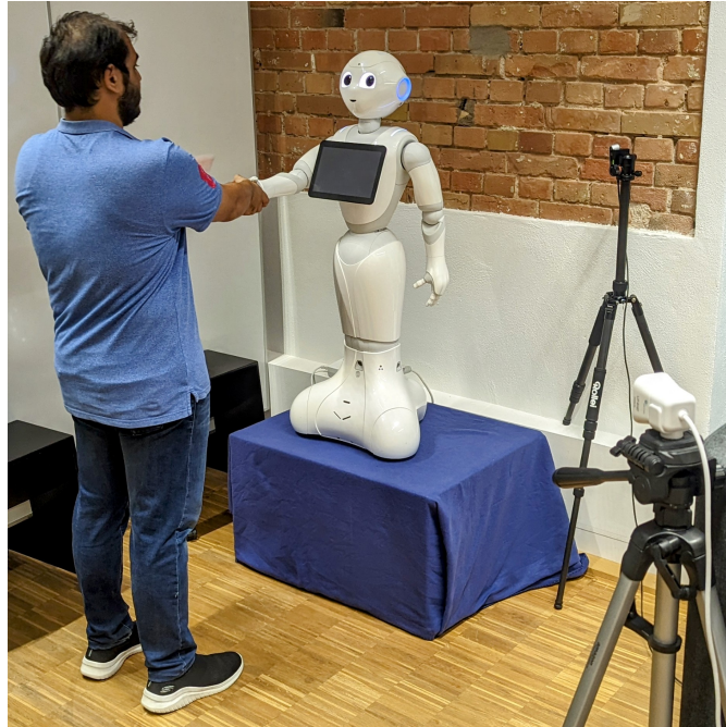
Figure 3.7.: Setup of the User Study for interacting with the Pepper robot. As Pepper is quite short (1.2m), it is placed on a pedestal to match the height of a human partner. The camera behind Pepper tracks the human partner's motion, which is used to generate Pepper's motions.
