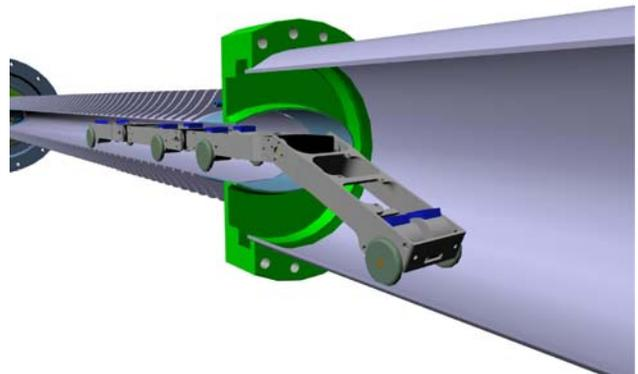
Figure 2: 3D simulation with the Gazebo [1] robotics simulator: A step is traversed as an example of a typical locomotion sequence of the inspection robot.
