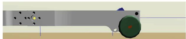
Figure 2: Sensor arrangement of the inspection robot indicated by the corresponding scanning beam directions.
