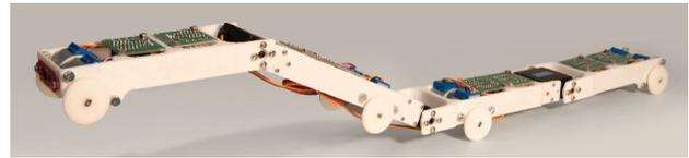
Figure 1: Prototype of the modular in-pipe inspection robot with 3D printed frames and wheels.
