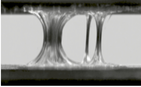
Figure 4.3: Side view of measurement with pronounced cavitation. Back cutting of finger formation leads to separation of liquid bridges. Measurement was performed with Gly80 , \lambda = 4 \times 10^{-5} and a = 180 \text{ m/s}^2 .
