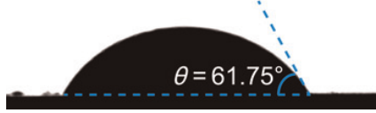
Figure 2.8: Contact angle measurement of distilled water applied to aluminium substrate.
