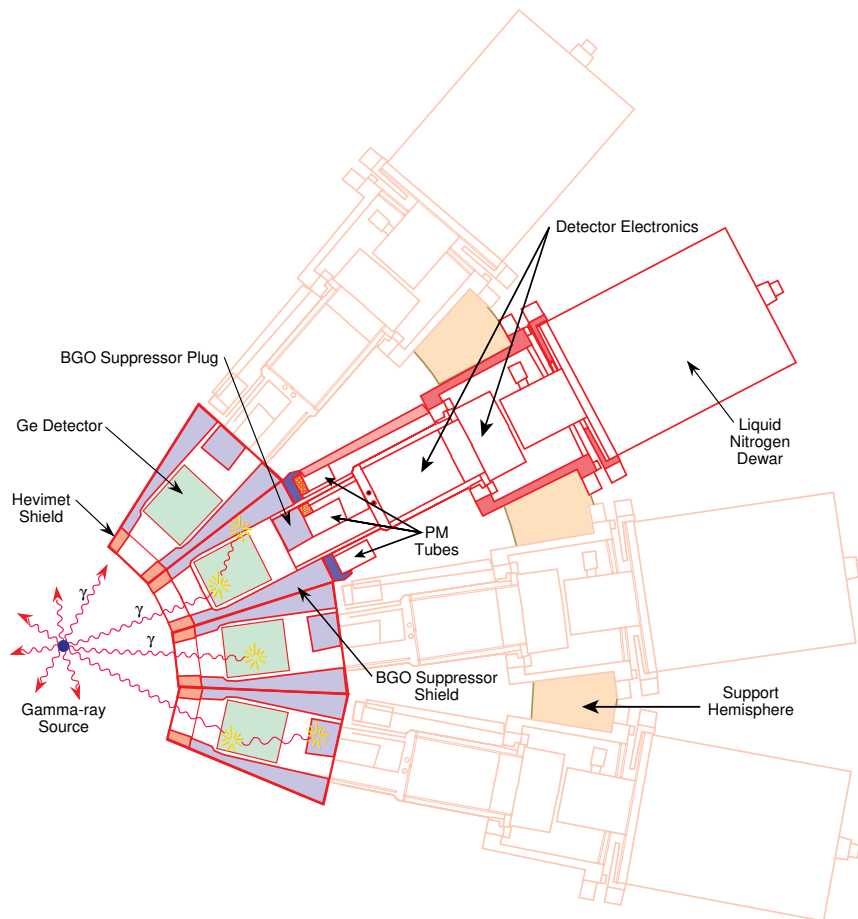
Figure 3.3: Sketch of four Gammasphere detector modules. Figure reprinted from [ES08] with permission from Elsevier.
