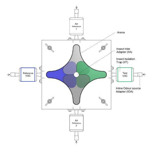
**Figure 1.** Top view of the four-chamber olfactometer. Insect arena is divided in four overlapping volatile organic compound (VOC) sectors, marked by colors. Arrows mark the connection to the clean air delivery system (CADS).
