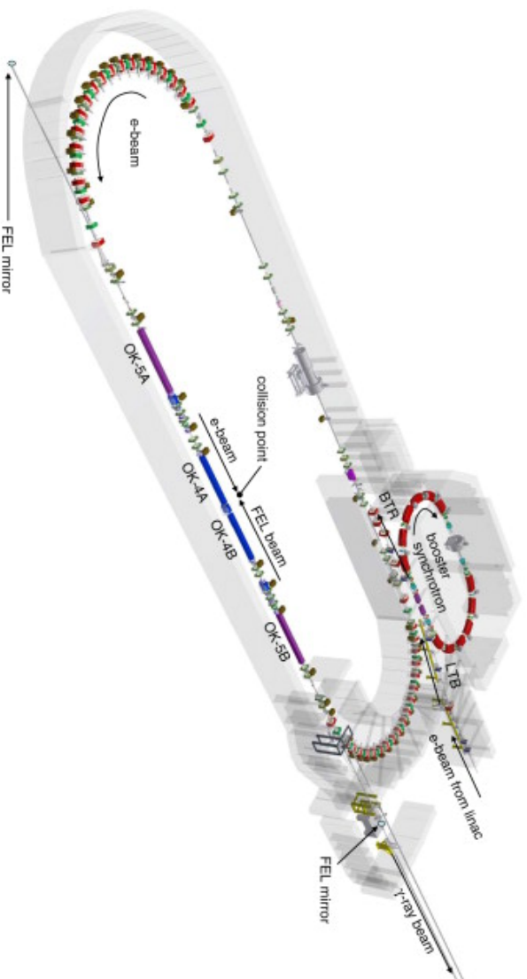
Figure 5.6.: Technical drawing of the HI \gamma S facility at TUNL. The Compton \gamma -ray beam is generated in the middle of the lower, long straight section (collision point) by colliding the electron beam with the FEL beam. The figure has been reproduced from Ref. [23], with permission from Elsevier Ltd. All rights reserved.
