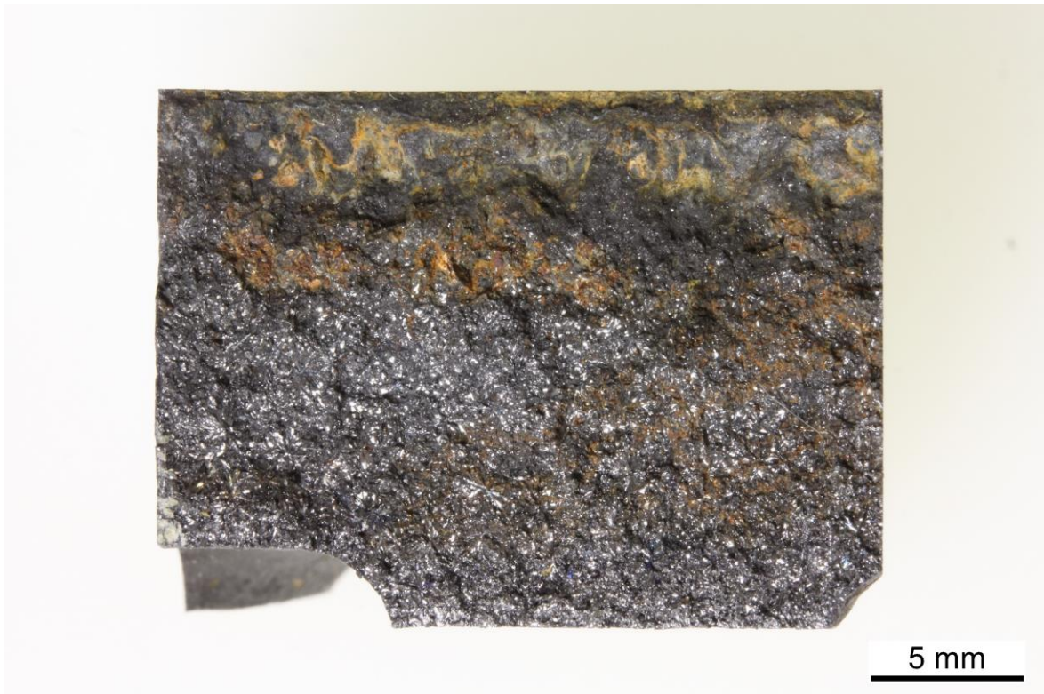
Figure 8-25: Opened through-thickness crack of the Reference brake disc
