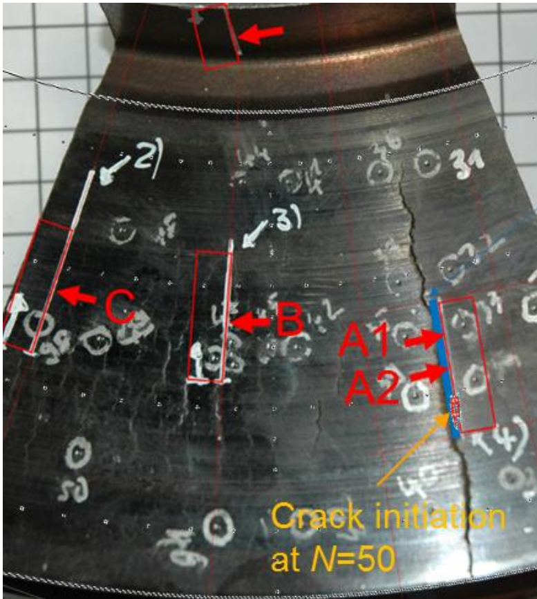
Figure 8-26: Photograph of the sampling segment for micrograph sections of the Reference brake disc; initiation point of the future through-thickness crack overlaid
