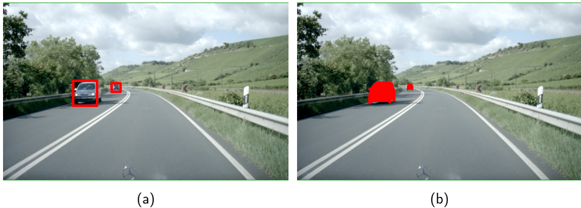
Figure 1.7: An image captured by a front mounted car camera with a resolution of 1024 \times 640 px with two front facing cars as objects. In 1.7a, the objects are described by bounding boxes (red rectangles) around the front appearance of the cars. In 1.7b, the objects are described by all pixels belonging to each object.
