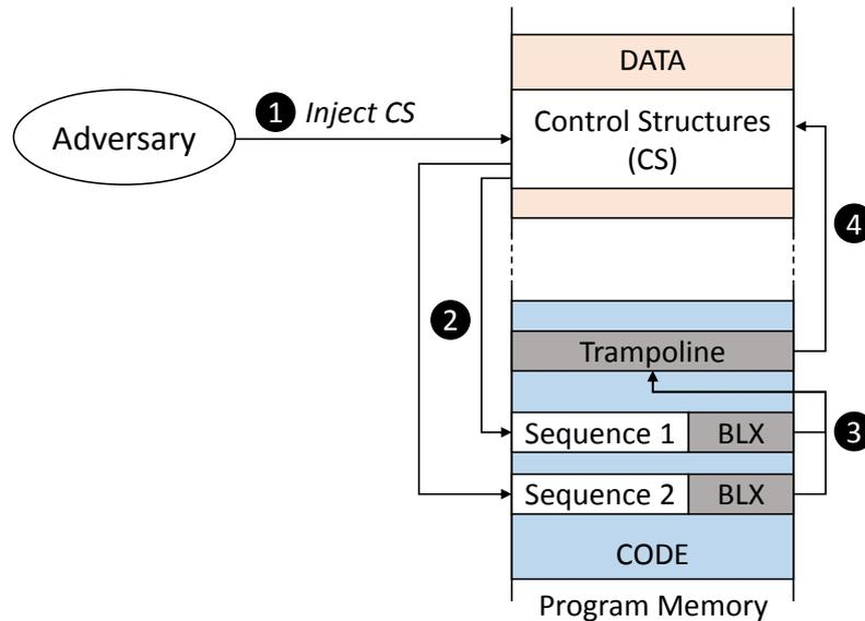
Figure 14: Basic layout of BLX-Attack on ARM
