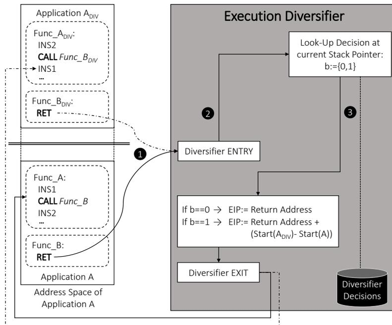
Figure 52: Instrumentation of function returns in ISOMERON
