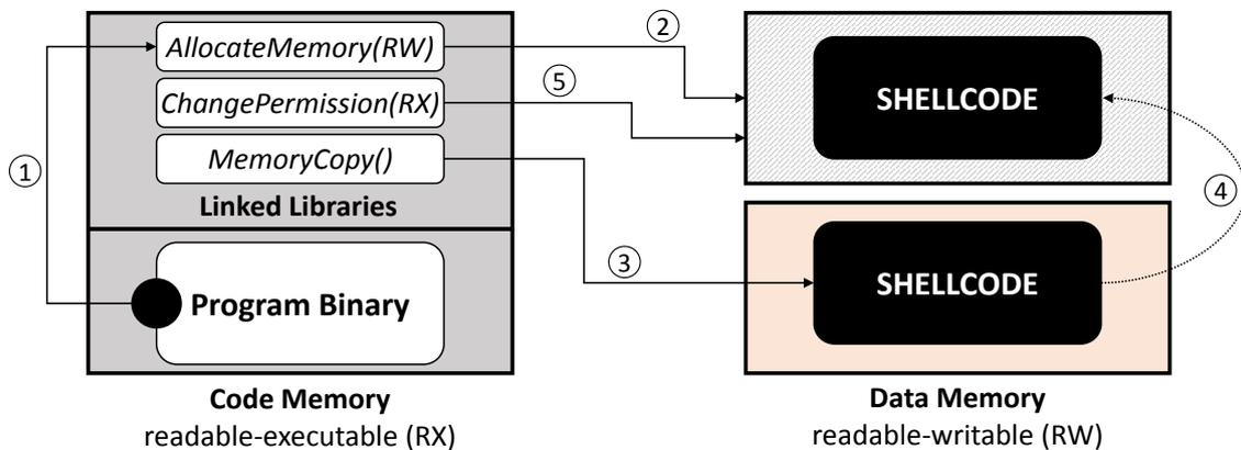
Figure 7: Hybrid exploitation: combination of code reuse with code injection
