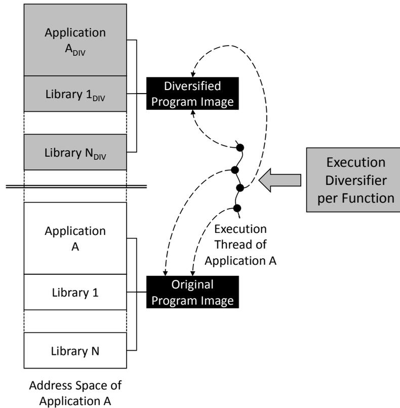
Figure 50: High-level approach to defeat traditional and just-in-time return-oriented programming attacks
