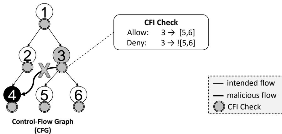
Figure 9: Control-flow integrity (CFI)
