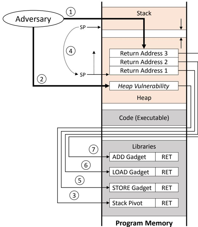
Figure 6: Basic principle of return-oriented programming attacks. For simplicity, we highlight a return-oriented programming attack on the heap using a sequence of single-instruction gadgets.
