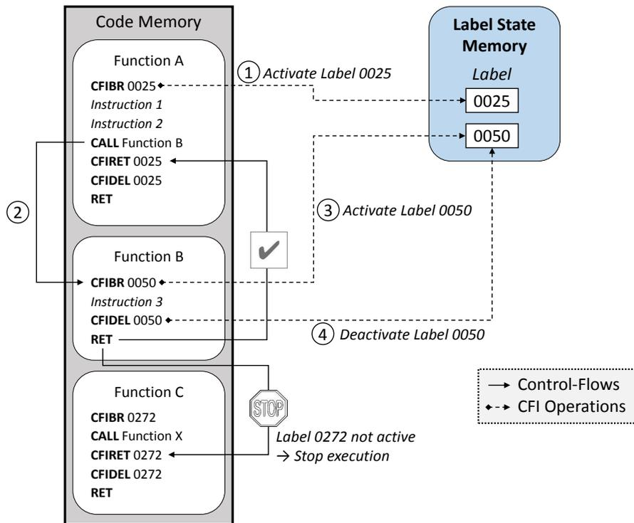
Figure 40: Workflow of call/return CFI checks in HAFIX
