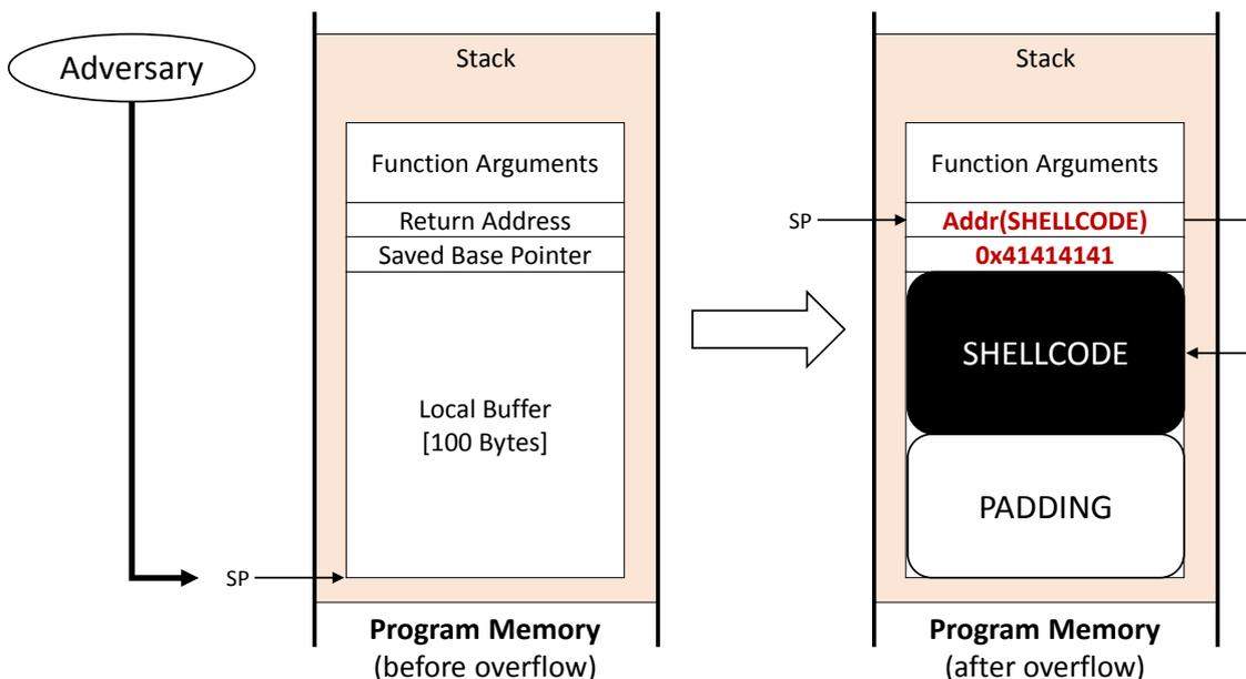
Figure 4: Memory layout of code injection attacks
