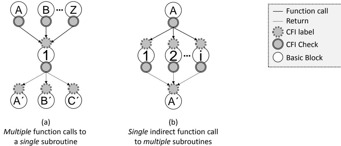
Figure 12: Static label-based CFI checks for function returns
