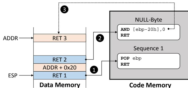
Figure 22: Details of NULL-Byte write gadget
