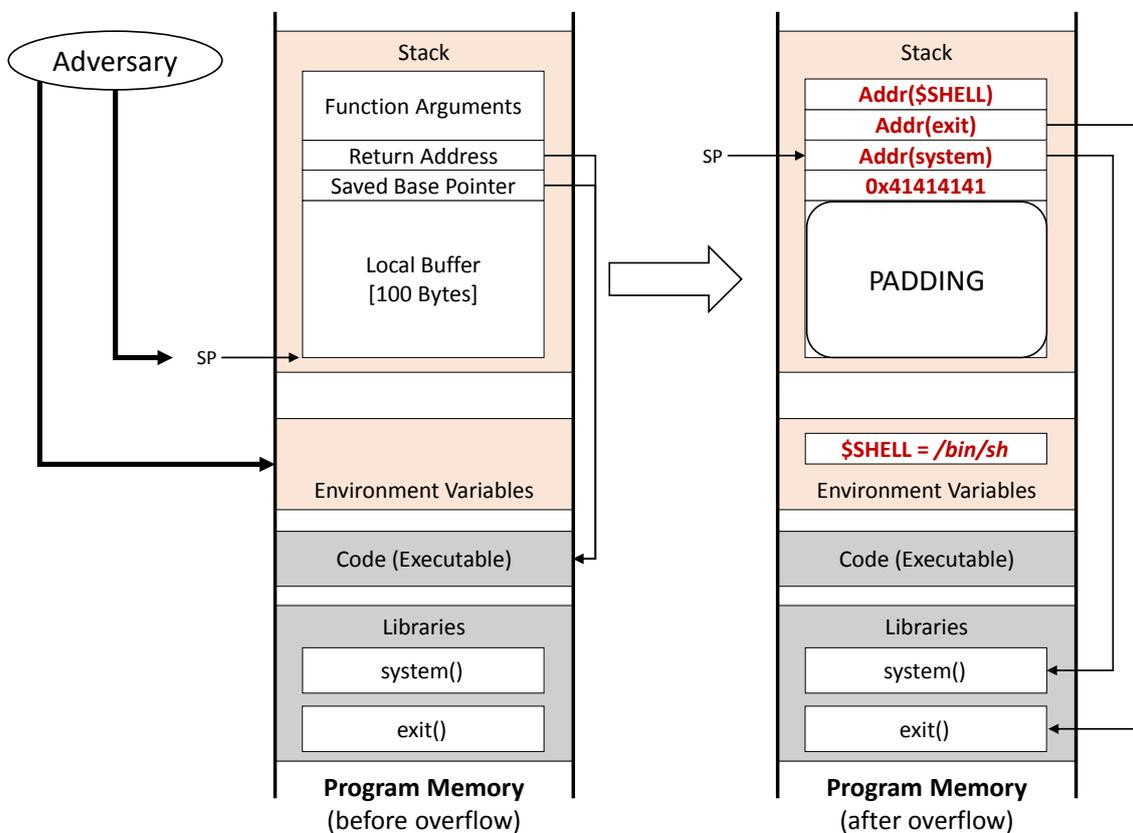
Figure 5: Basic principle of return-into-libc attacks
