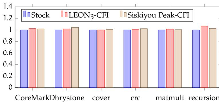
Figure 42: CFI extension overhead w.r.t stock core for LEON<sub>3</sub> and Siskiyou Peak
