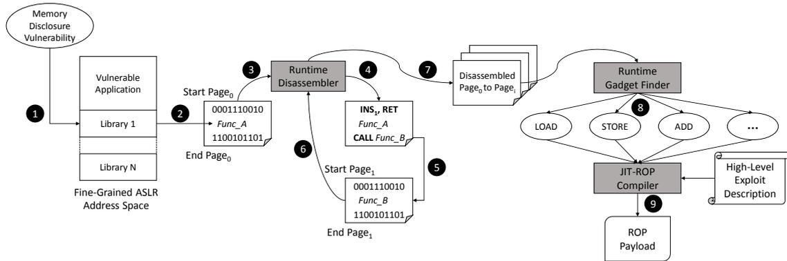
Figure 49: Workflow of a JIT-ROP attack
