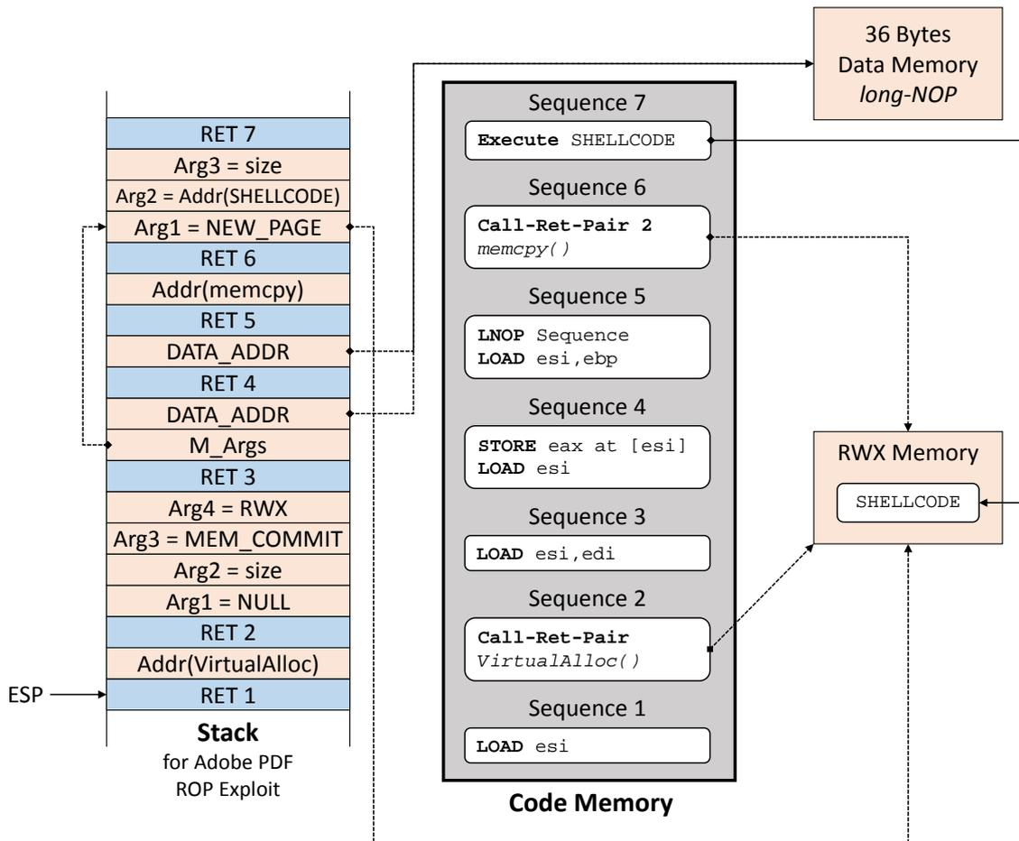
Figure 24: Simplified view of our hardened PDF exploit. See Appendix in [65] for the full source code.
