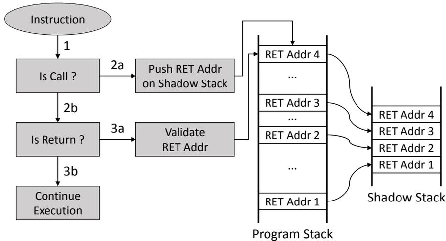
Figure 13: Main principle of shadow stack (return address stack)
